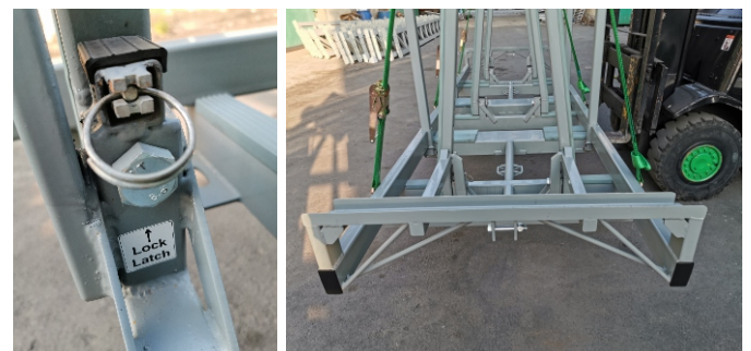
Pull lock latch out & twist to fold-down 'A's
