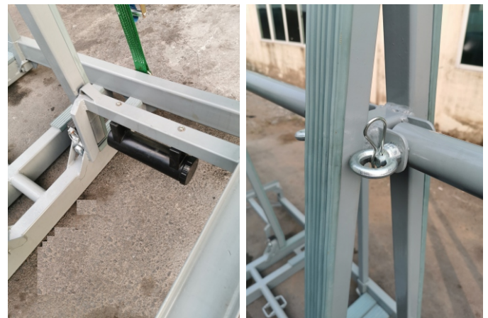
Document Container (Manual) & Eye Nut & Release Pin
